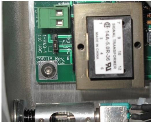
Figure 3-4: Voltage selection header (shown 220VAC, pin2-3)
