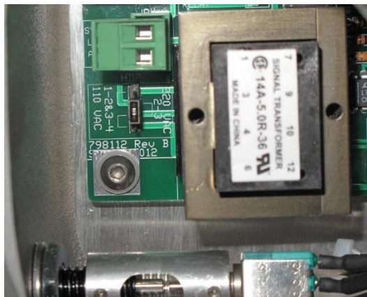
Figure 3-6: Voltage selection header (shown 220VAC, pin2-3)
