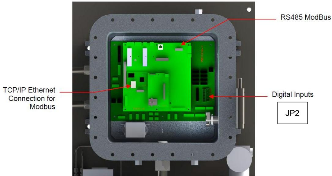
Figure 4-8: Upper Control Enclosure - Modbus and Digital Inputs
