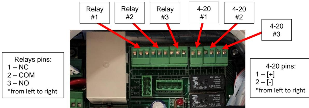
Figure 4-6: Analog 4-20 mA and Relays Output Connections
