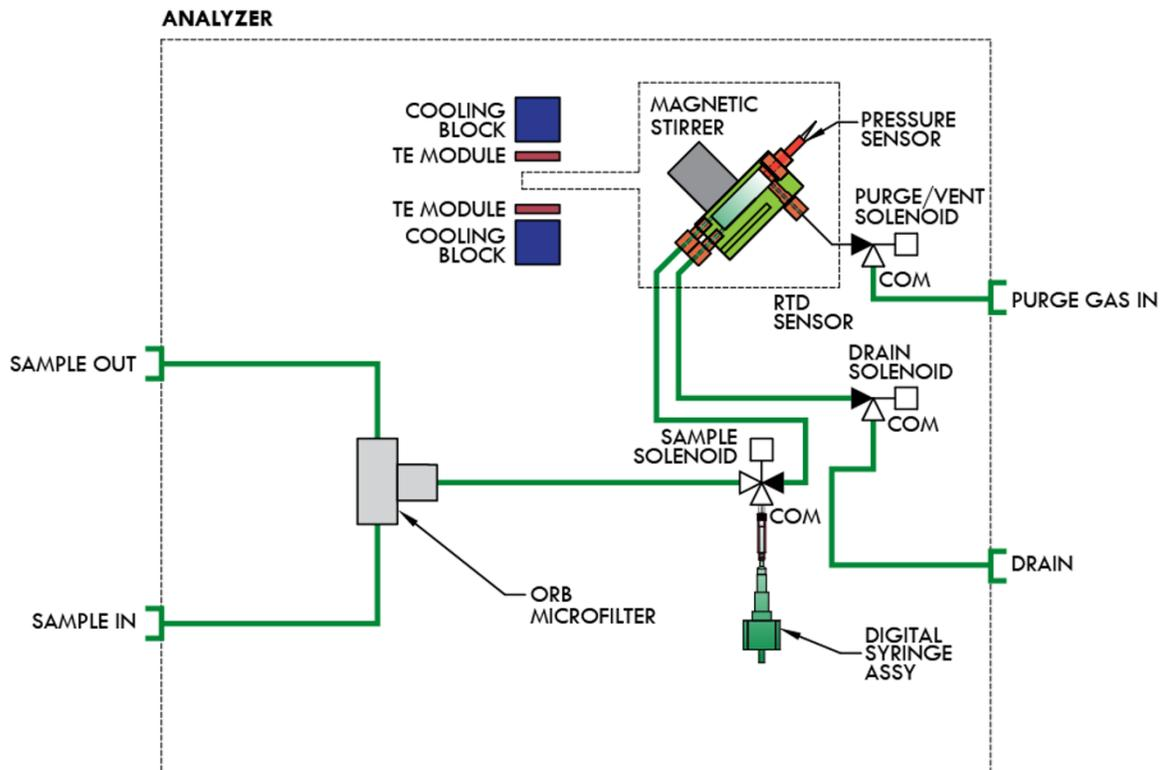
Figure 1-1: Analyzer Flow Schematic
