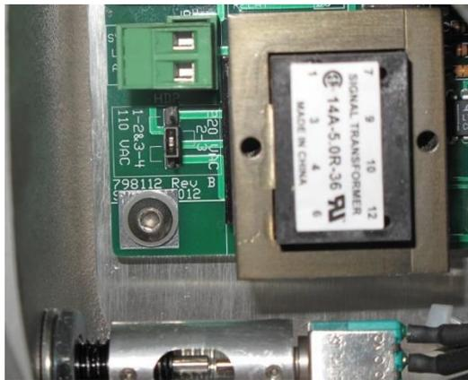
Figure 4-4: Voltage selection header (shown 240 V a.c., pin2-3)
