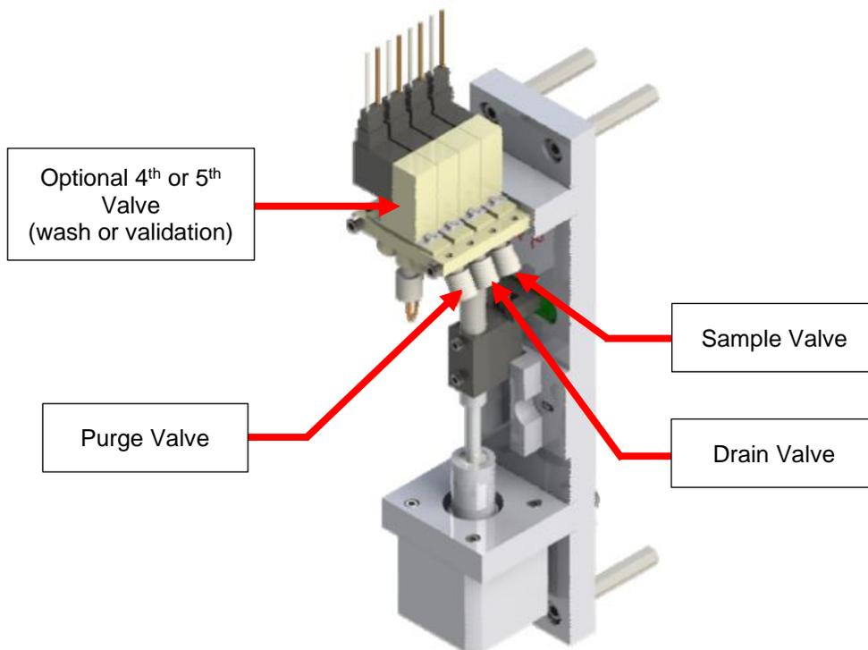
Figure 7-2: Solenoid valves location
