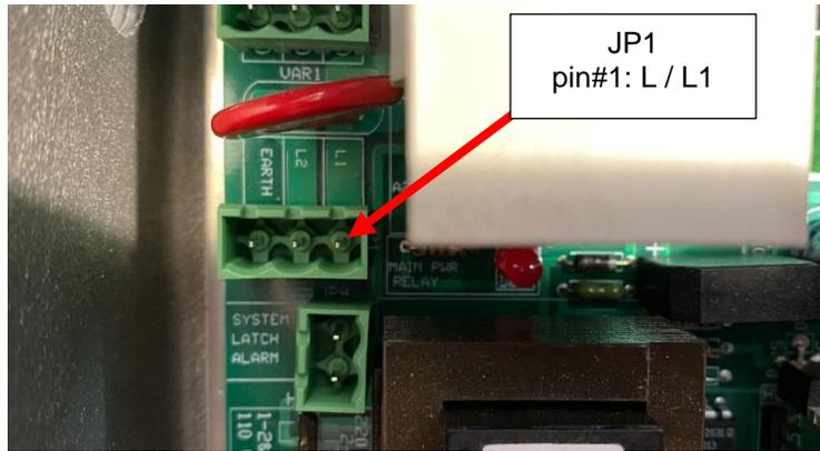
Figure 4-5: Customer Power In on JP1 header
