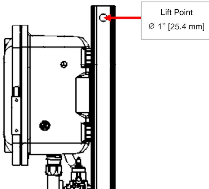
Figure 4-1: Lifting Point Location
