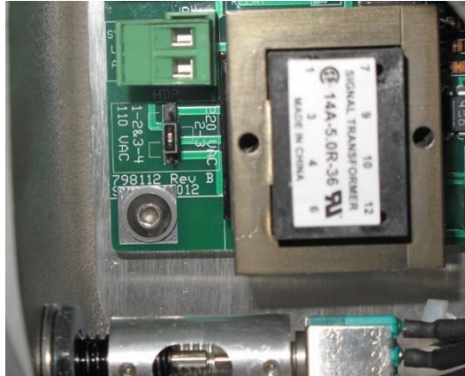
Figure 4-4: Voltage selection header (shown 240 V a.c., pin2-3)
